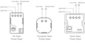
Please connect according to the actual marking on the product Stripping length 10mm L: Live wire input N: Neutral wire input
